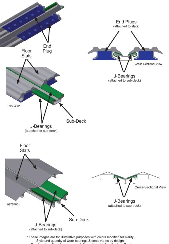
Wear bearings & seals are non-metallic and run the length of the floor. (They are designed to be replaced to extend the life of the floor.)
